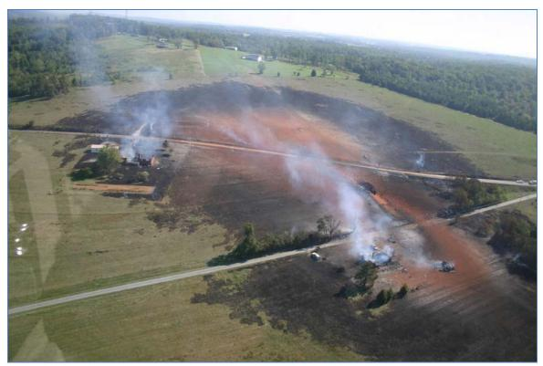
Figure 2 – Example of Damage Caused by Hitting Gas Line (out-of-state contractor not associated with this project)
