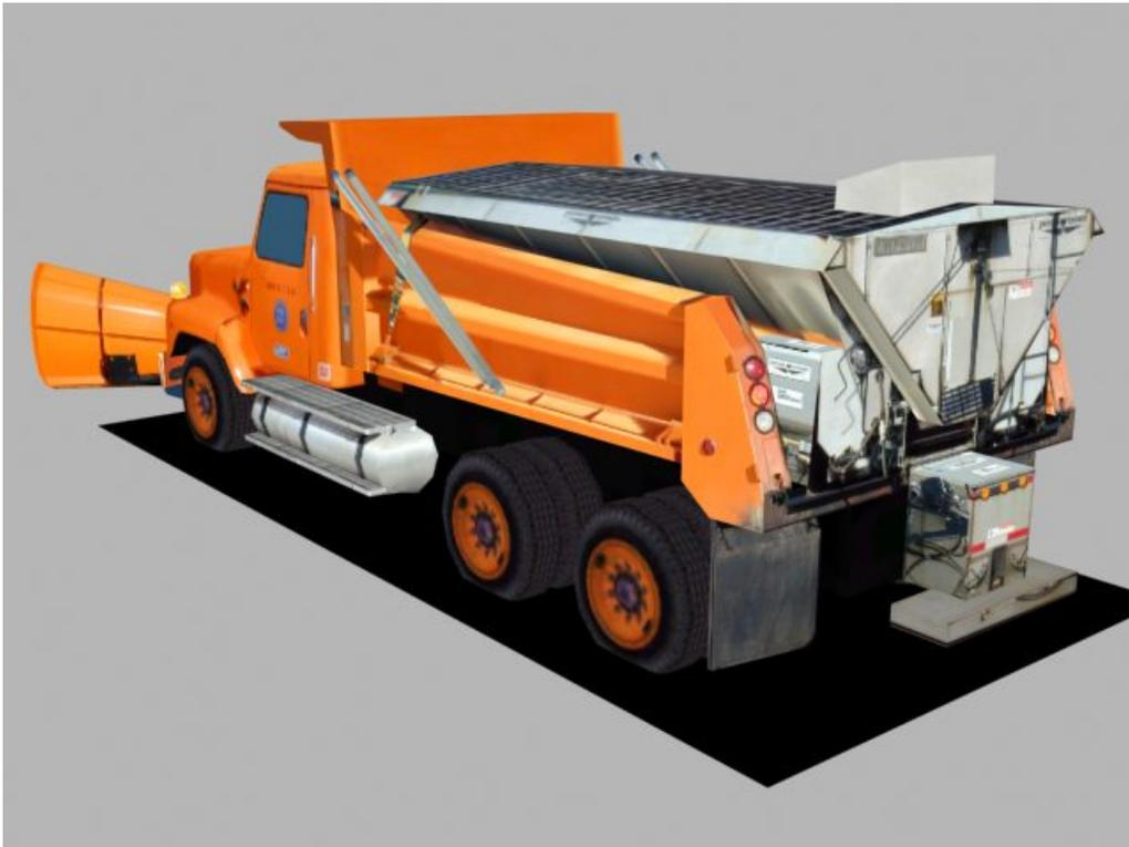
Figure 6. Rear view of the simulated snowplow
