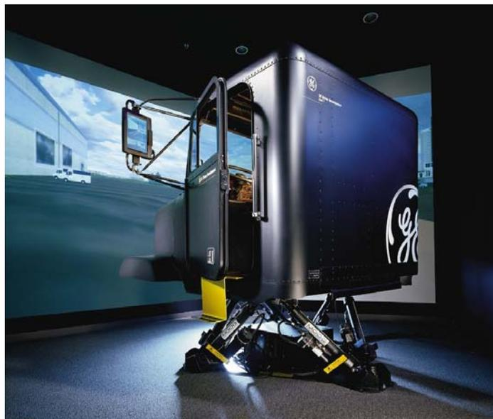
Figure 2. The Mark II motion-based simulator
