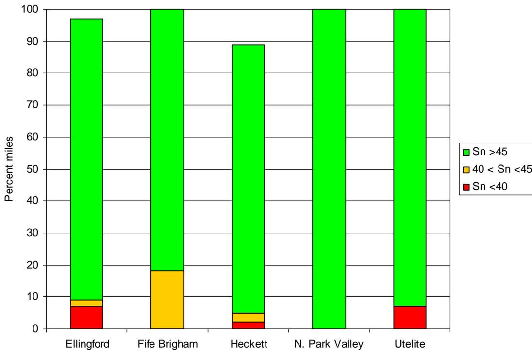
Figure 8. Effect of aggregate source on skid resistance of CSC
