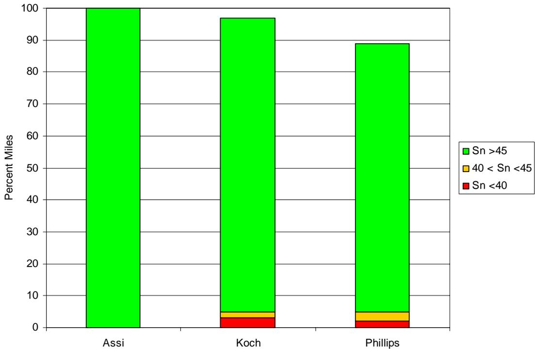
Figure 10. Effect of asphalt binder source on the skid number of CSC
