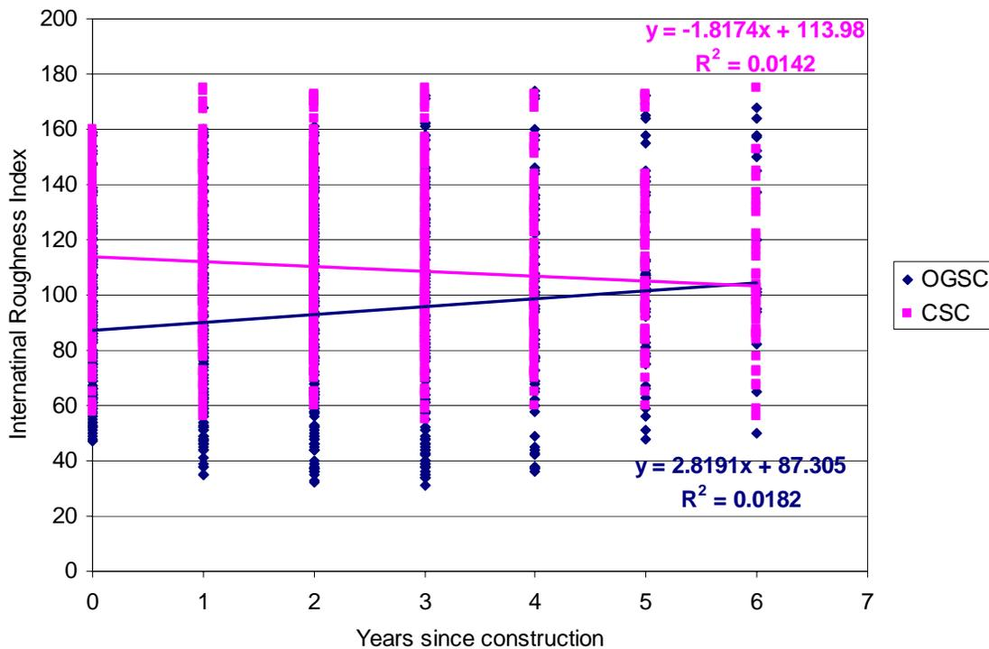
Figure 2. Roughness index for all sections evaluated
