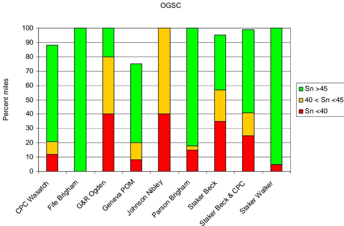
Figure 7. Effect of aggregate source on skid resistance of OGSC
