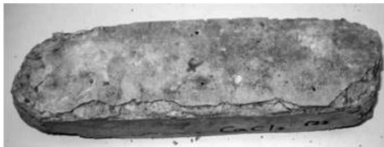
**Figure 3-5 Specimen following 10 weeks of exposure to 6.04 molal ion concentration of CaCl<sub>2</sub> (56).**
