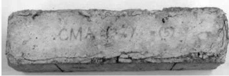
**Figure 3-11 Specimen following 95 weeks of exposure to 1.06 molal ion concentration solution of CMA (56).**
