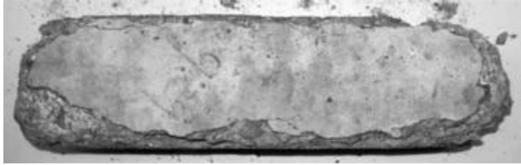
**Figure 3-6 Specimen following 10 weeks of exposure to 6.04 molal ion concentration solution of  $\text{MgCl}_2$  (56).**
