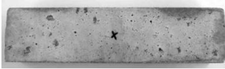
**Figure 3-8 Specimen following 95 weeks of exposure to 1.06 molal ion concentration solution of NaCl (56).**
