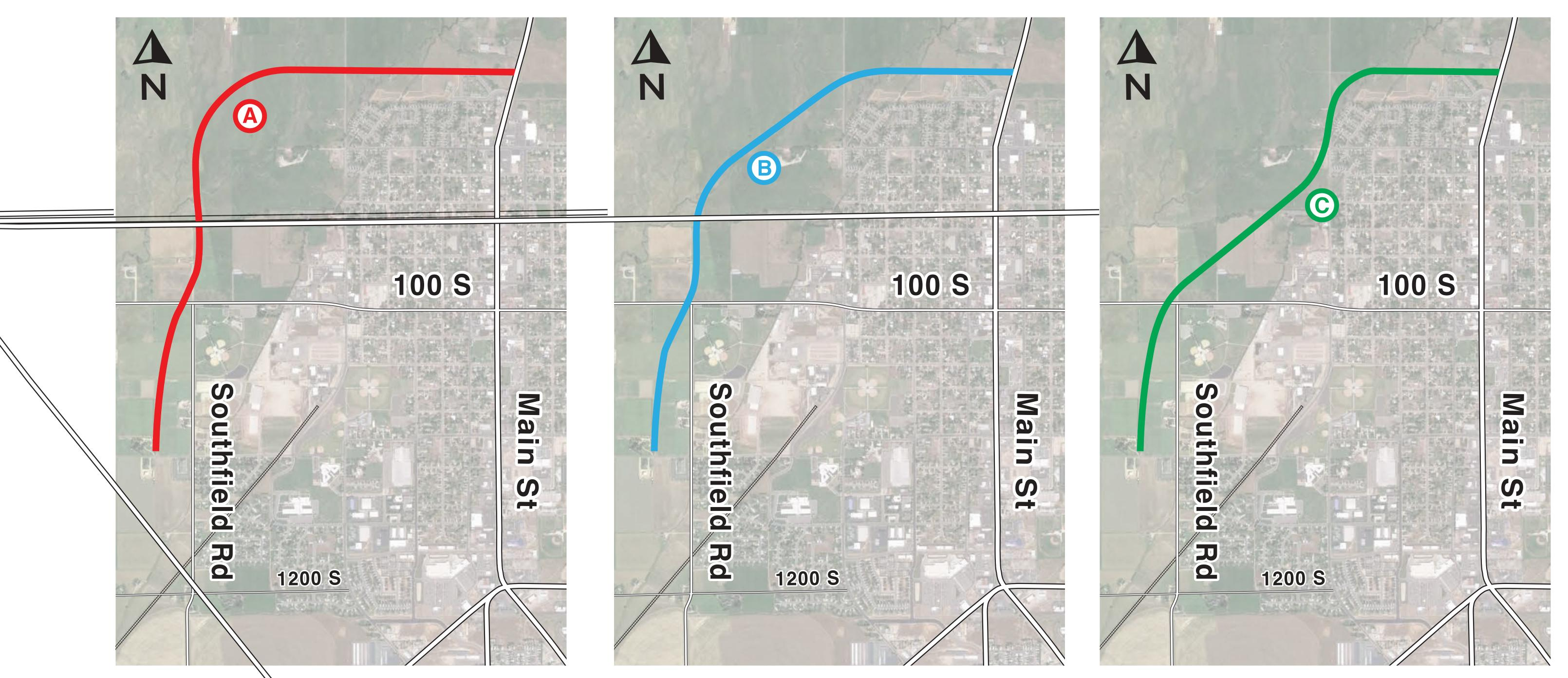
Three options were reviewed for the northern segment. Due to extensive wetlands, further evaluation is needed in an environmental study to determine a recommended route for this area.
