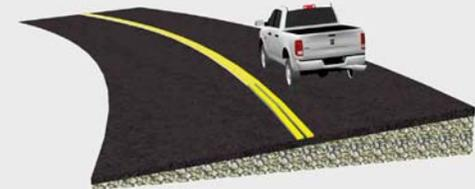
**Example of superelevation of road**
